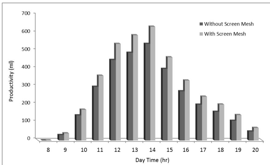
Figure 10. Hourly variation of the still productivity for air velocity of 0.9 m/s with and without present of the screen mesh
