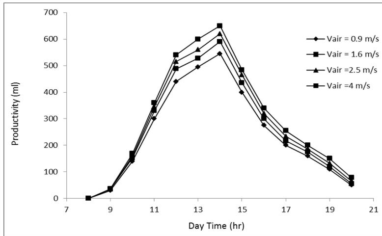
Figure 8. Hourly variation of the solar still productivity for different air velocity.
