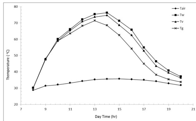
Figure 6. Hourly variation of the solar still temperatures for air velocity of 4 m/s.
