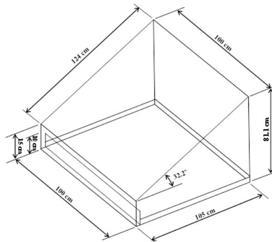
Figure 1. Isometric view of the experimental setup.
