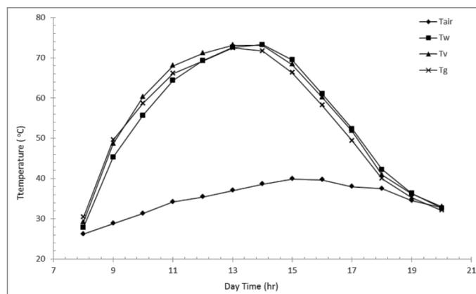
Figure 3. Hourly variation of the solar still temperatures for air velocity of 0.9 m/s.
