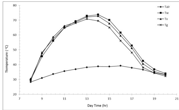
Figure 4. Hourly variation of the solar still temperatures for air velocity of 1.6 m/s.
