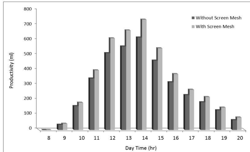
Figure 11. Hourly variation of the still productivity for air velocity of 2.5 m/s with and without present of the screen mesh
