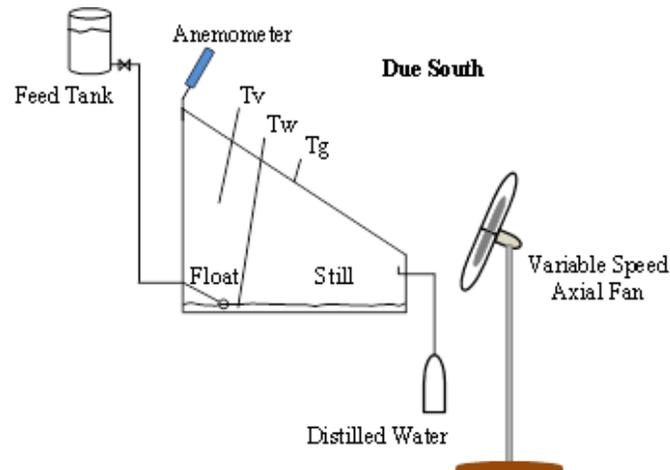
Figure 2. The solar still overall schematic diagram.
