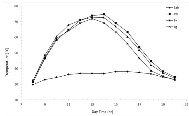
Figure 5. Hourly variation of the solar still temperatures for air velocity of 2.5 m/s.
